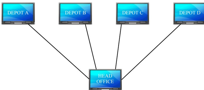
If depot's A, B, C & D wish to send their data to Head Office only, the 'Remote Server Settings' on all four depot's computers will be identical, i.e the remote server details on each depot computer will be that of the head office computer. No remote server details need to be entered on the head-office computer, but the Internal Server Settings must be Enabled.
