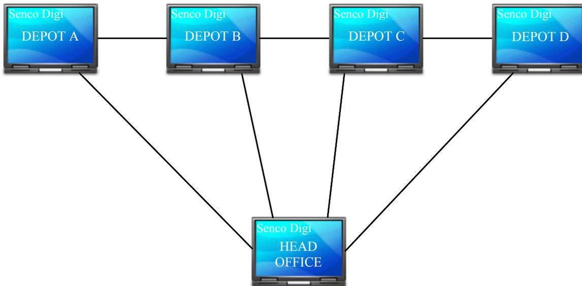
The software contains an inbuilt networking system for the transfer of downloaded driver card data between any number of computer terminals that have Senco Digi installed. It operates seamlessly in the background with no user intervention required (after initial setup) over both Local Area Networks (LAN) or Wide Area Network (WAN) or a combination of both.
